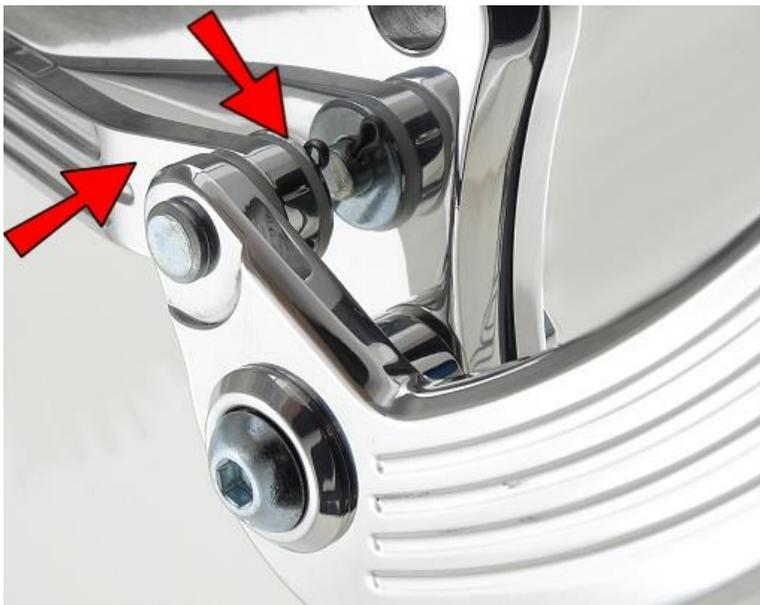
Place the Brake Linkage Extension onto the Clevis Pin, then place another 3/8" Nylon washer onto the Clevis Pin, then a 1/4" Zinc washer and secure with a 5/64x1 Cotter Pin.
