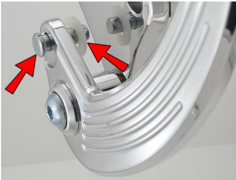
Insert a 5/16x7/8 Clevis Pin into the Brake Pedal, then place a 3/8" Nylon washer onto the Clevis Pin.
