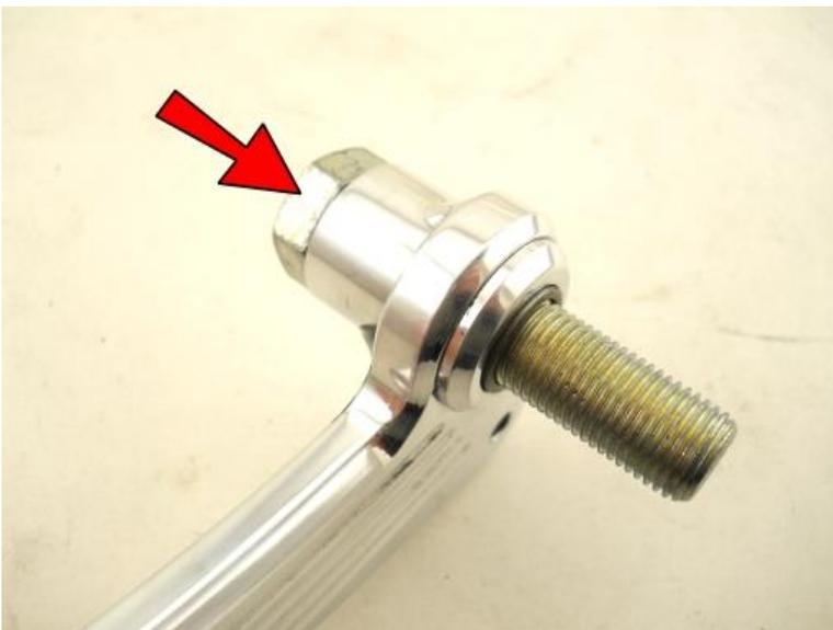
Place a 1/2" Washer onto the Bolt on the front side of the Shifter Pedal.
