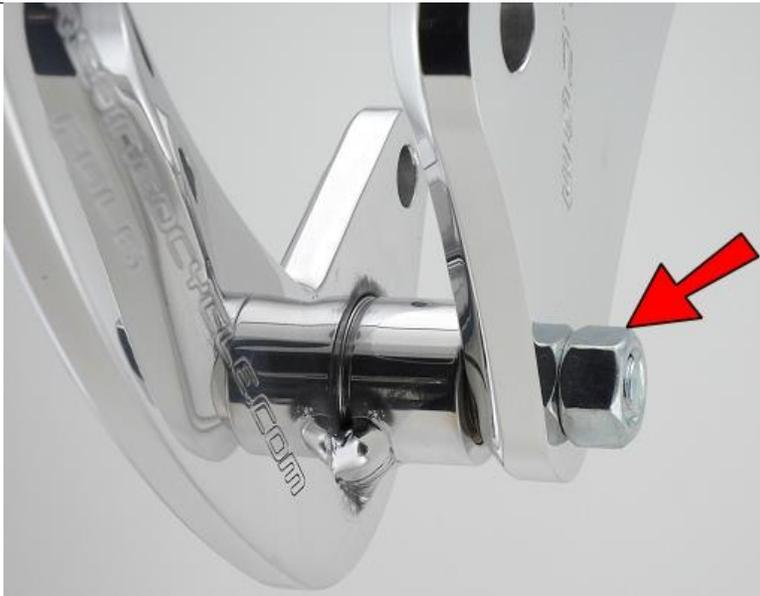
Connect the Brake Pedal to the FC1-R and secure with a 3/8" Nut.
