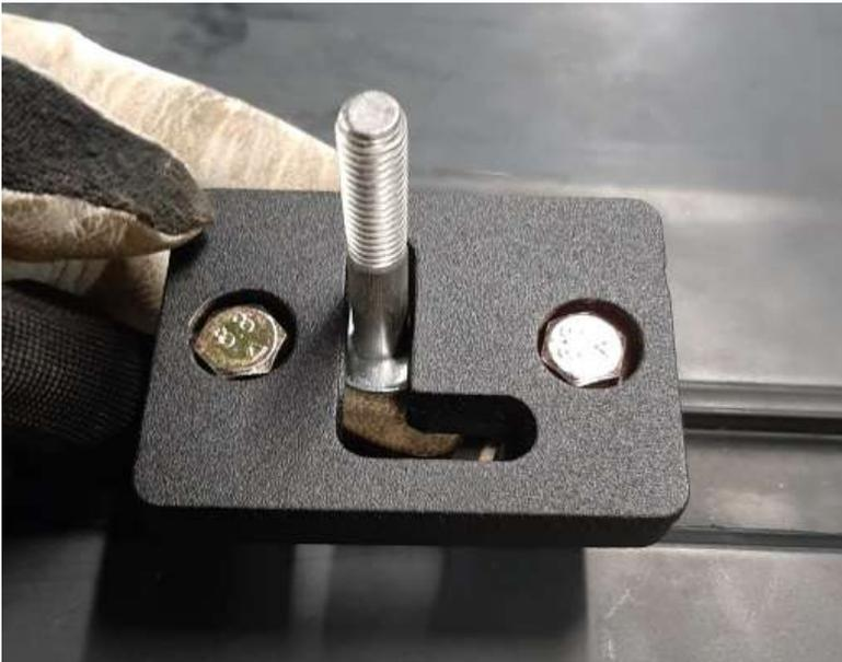
Insert the 3/8 Bolt into the plates from underneath and hold it in position.
