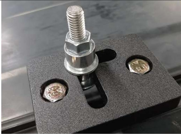
Thread on a 3/8 Nut leaving it loose enough so that you can still slide the Bolt in the slot.
