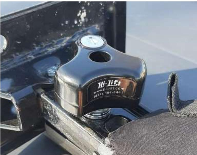
The use of a locking knob such as Hi-Lift part# HM-LK is highly recommended to secure your Hi-Lift Jack.
