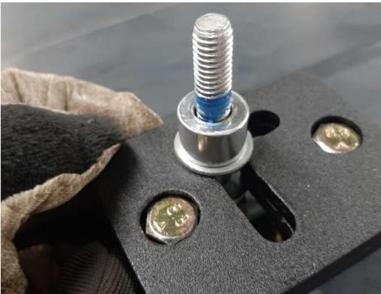
Place another Washer and .5" Spacer onto the Bolt and apply some thread-lock where the nut will go.
