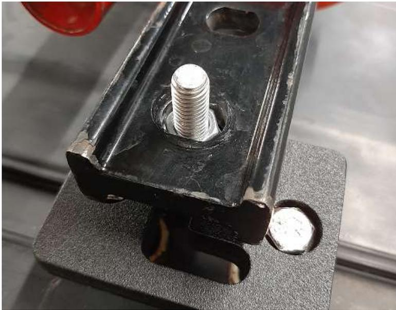
Now slide the 3/8 Bolts to align with the closest holes in both ends of the jack and place the jack onto the 3/8 Nuts. (Notice the flats of the holes should align with the flats of the Nut)
