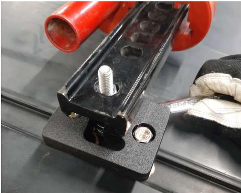
The jack will hold the Nut so that you can use a wrench on the 3/8 Bolt head and tighten. You may want to remove the jack and use wrenches on both to do a final tightening of the 3/8 Nut on the 3/8 Bolt.
