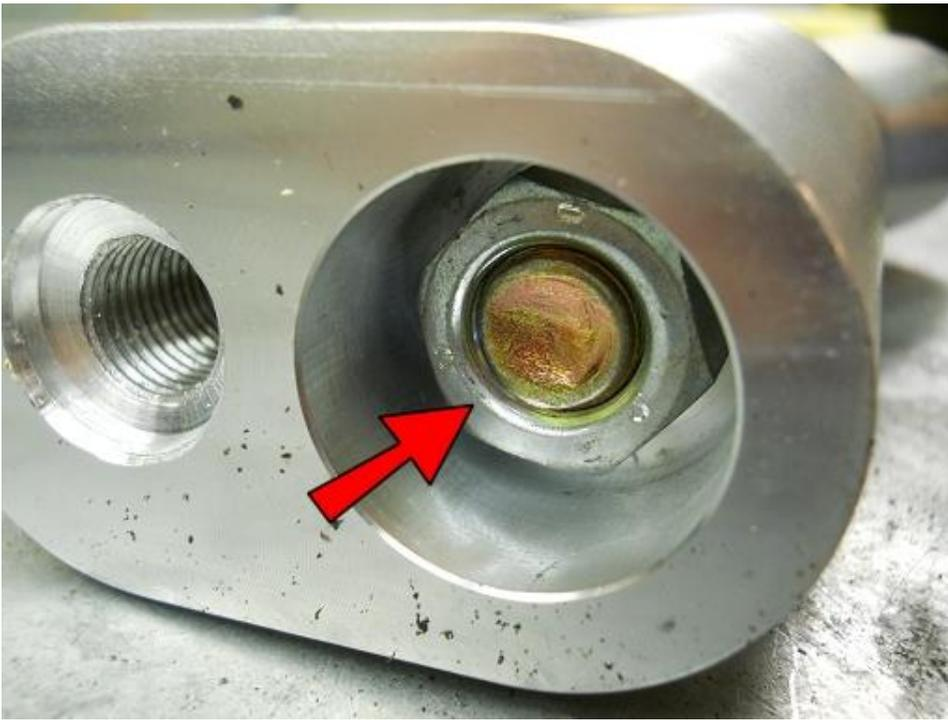
Connect both risers to the HR3's and thread on a 1/2-20 nut. Only tighten it enough to loosely snug them together allowing you to center the rubber washer that now sits between the riser and HR3.
