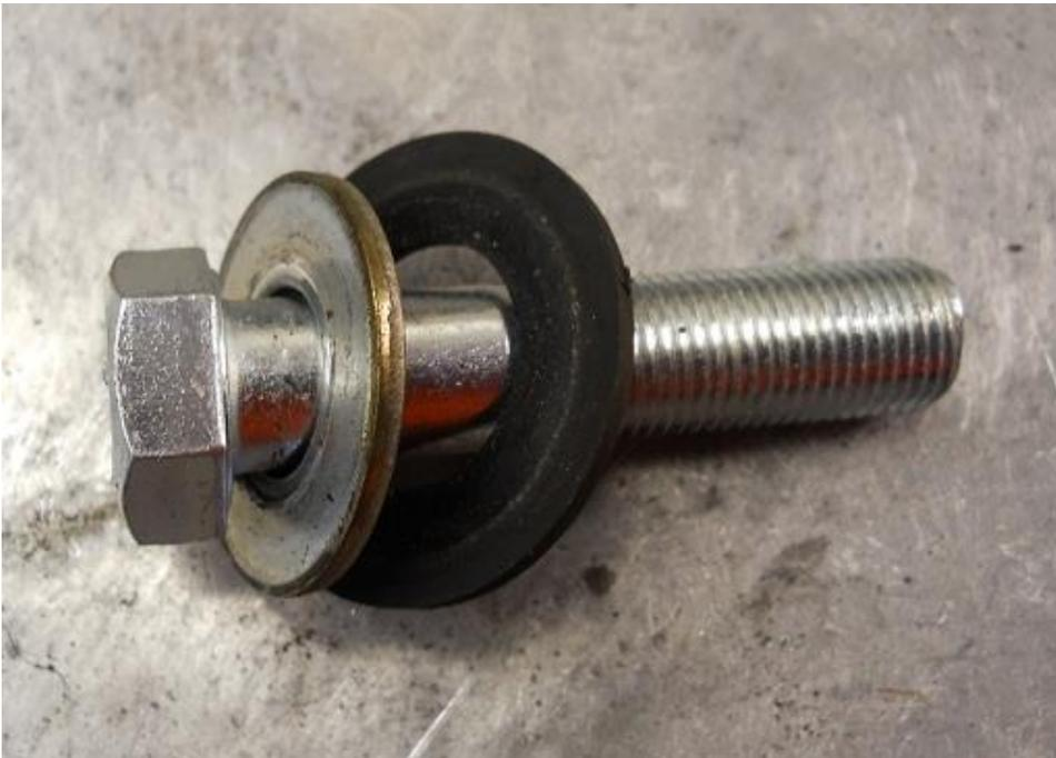
Place the other zinc washer and rubber washer onto 1/2-20x2.25" bolts.
