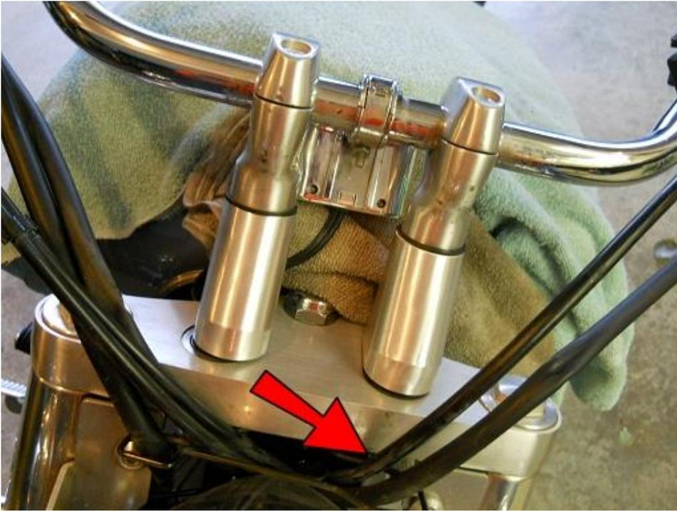
Attach one of the risers to the triple tree with a 1/2-20x2.25" bolt that you just put the washers onto. Only finger tighten at this point. Don't worry if the other side doesn't line up right now.
