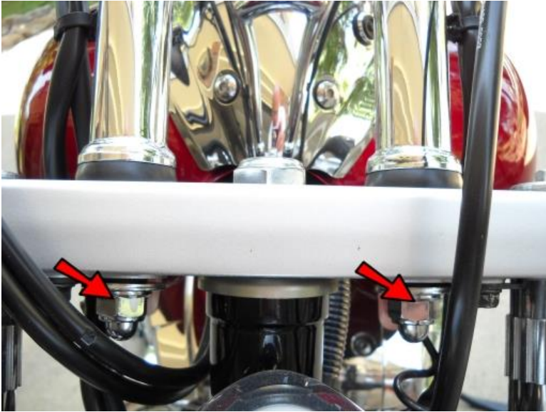
Remove these two nuts and washers to remove the handle bars.
