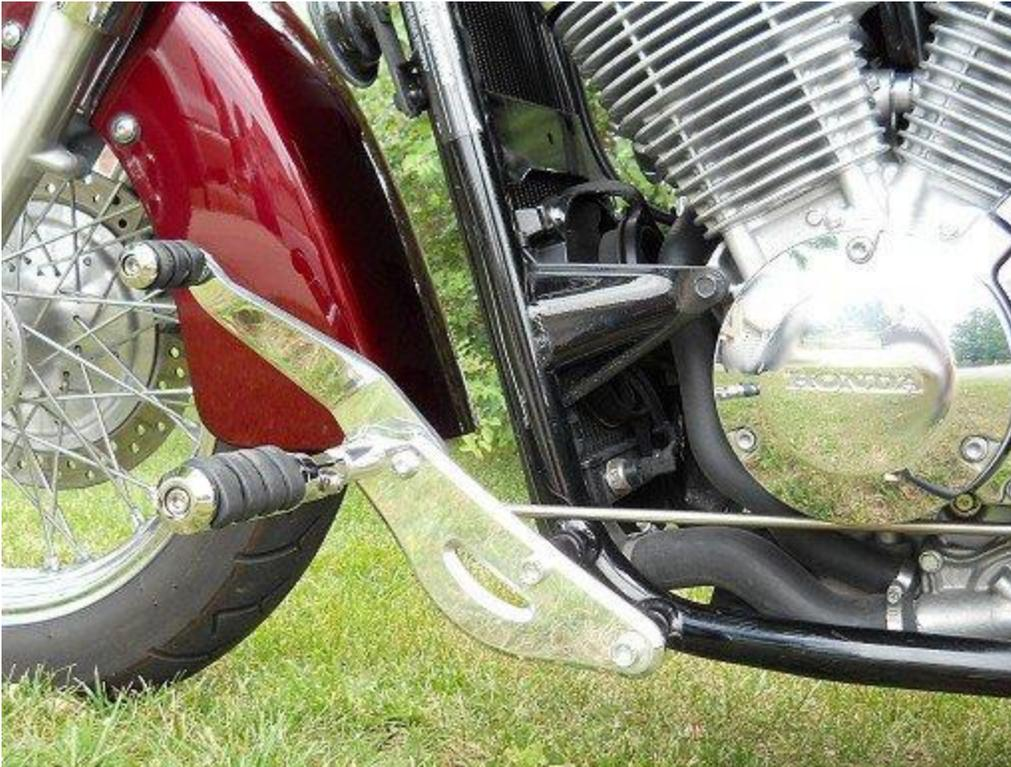
Test the Shifter Pedal for desired position. To make a small adjustment, rotate the shifter linkage a few turns, but make sure there is still most of the thread, threaded into the rod ends. If more adjustment is necessary, remove the bolt from the shifter arm shown in picture K, and remove the arm from the spline. Rotate the arm 1 or 2 notches in the direction you want the shifter pedal to move and reconnect.
