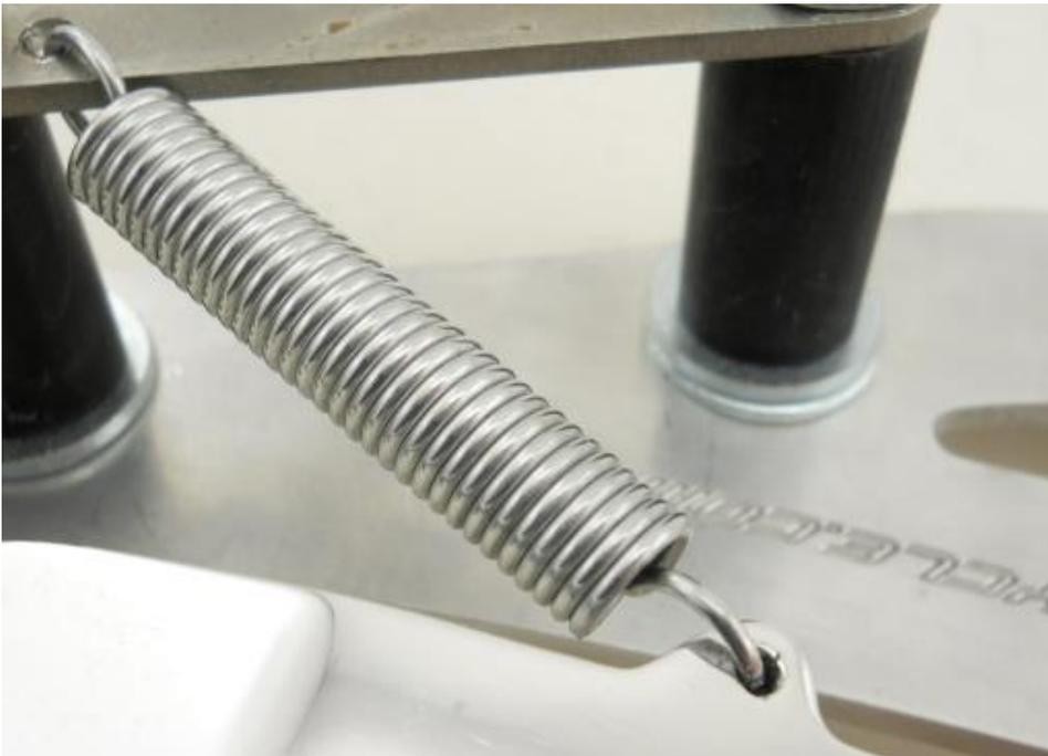
Hook one end of the spring into the small hole in the BSM2 and the other end of the spring into the small hole in the Brake Linkage.
