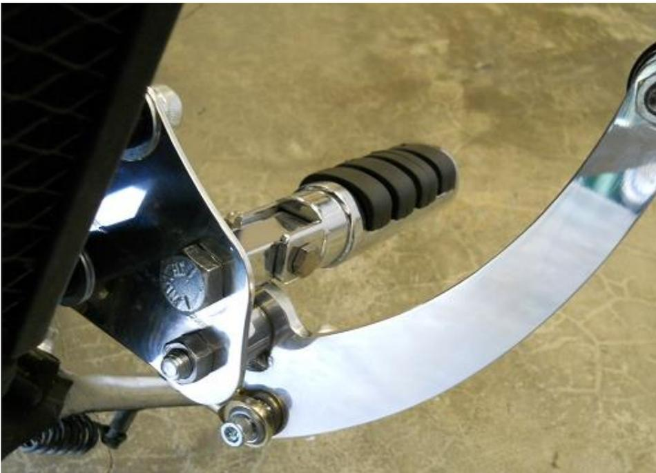
Install a foot peg into the top hole of the FC6-L. Connect the Shifter Pedal to the outside of the FC6-L with a 3/8-16x2 Button Head Bolt and secure with a 3/8 nut. Attach the other end of the Shifter Linkage to the Pedal with an M6-1.0x25 Bolt and secure with an M6 Acorn Nut on the front.
