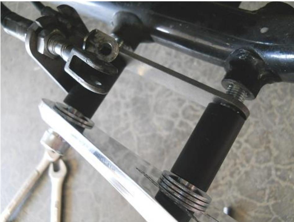
Insert an M10-1.25x70 bolt into the bottom holes of the FC6-R. Place one 3/8" Washer onto the back bolt and two 3/8" Washers onto the front bolt as shown. (If it looks like more washers, that's just a reflection.) Place the 1.5" Spacers onto the bolts, line the bolts up with the holes of the BSM2 and thread into the frame and tighten. You may need to work some slack in the cables to get it all to line up. This is why you previously loosened them.
