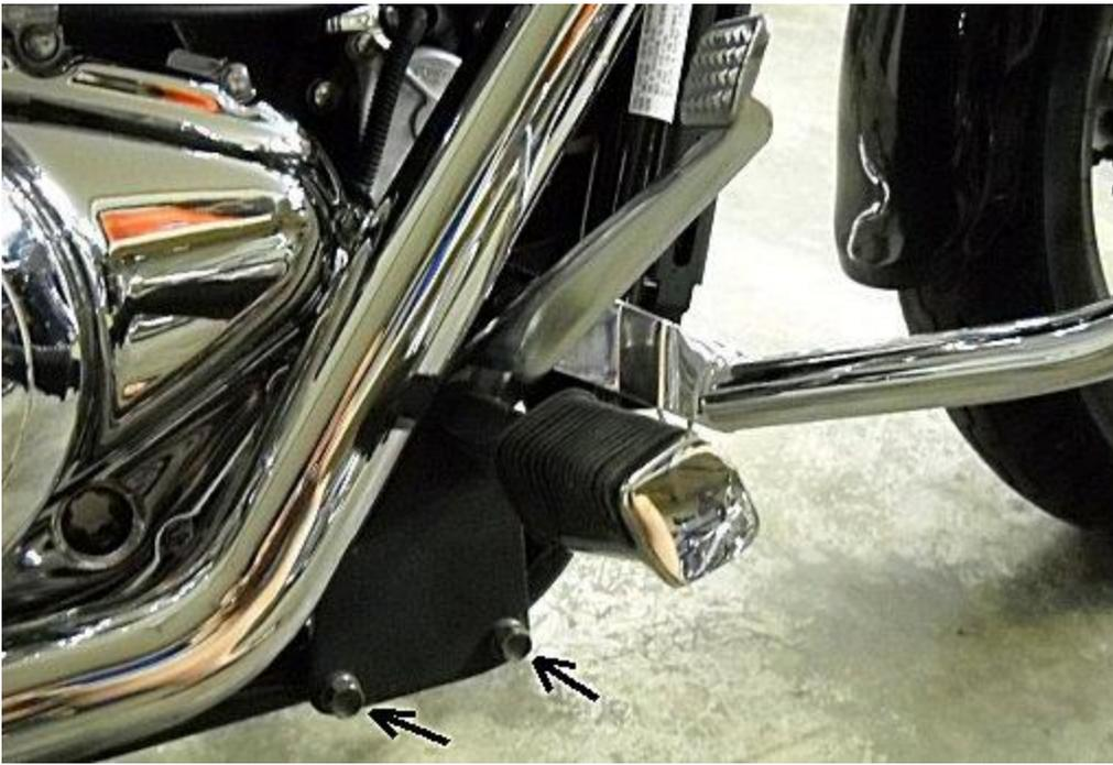
On the brake side, remove the stock foot control bracket by removing the two 10mm bolts attaching it to the frame.
