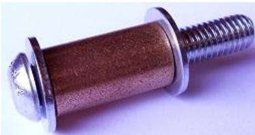
**NOTE:** If you are using a 3/8" mounted foot peg, the shifter will mount much like the brake side, with the alternate hardware arranged as shown here, NOT as shown below with a 1/2" bolt. (Make sure the smaller, steel sleeve is inside the bronze sleeve.)
