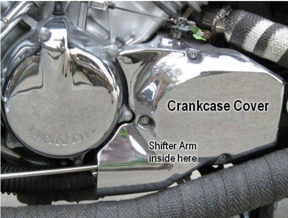
Remove the stock shifter linkage from the ball joint at the shifter arm under the chrome crankcase cover by rotating the linkage clockwise (it is a left hand thread).
