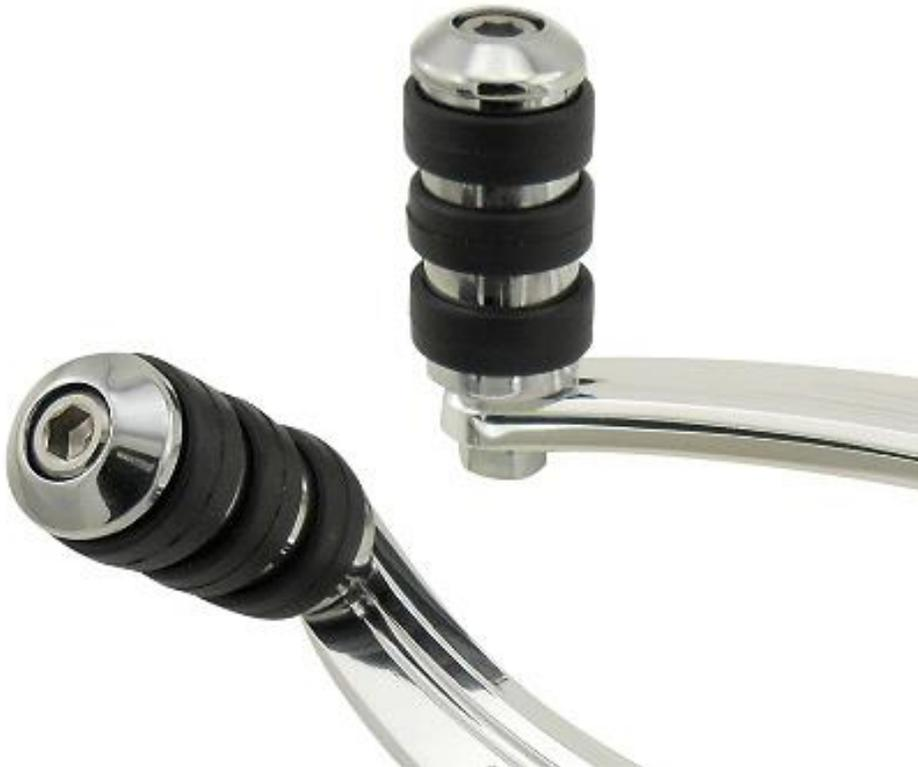
Attach the Toe Pegs to the threaded top hole of the Shifter and Brake Pedals and secure with a 5/16" Nut.
