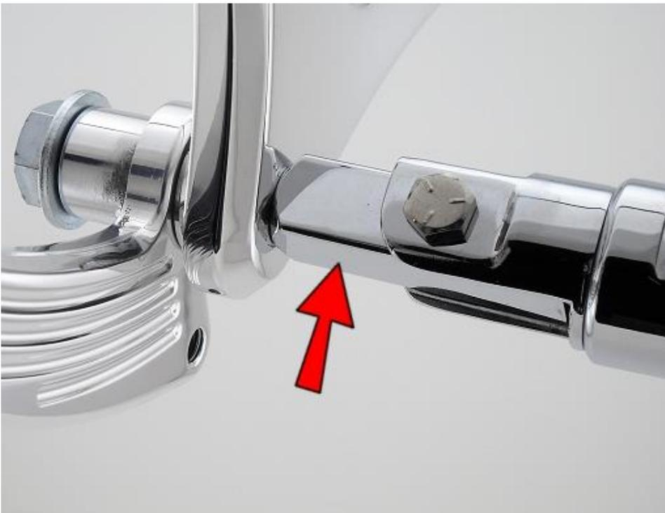
Thread the foot peg onto the 1/2-20x2.25 Bolt and tighten in the desired position.
