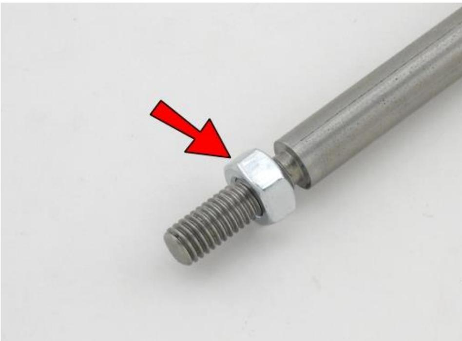
Remove the nuts from both ends of the stock linkage and thread them all the way onto the new Shifter Linkage. (Make sure to put the left hand threaded nut onto the correct end.)
