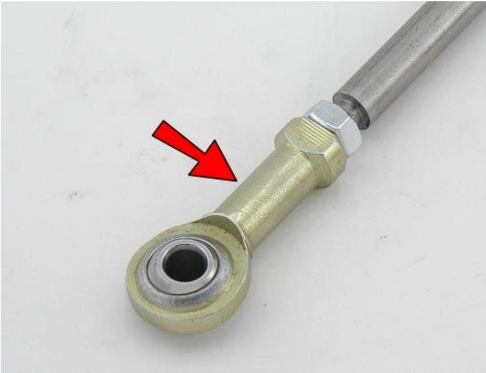
Connect the M6-1.0 Spherical Rod End to the right hand threaded end of the Shifter Linkage.
