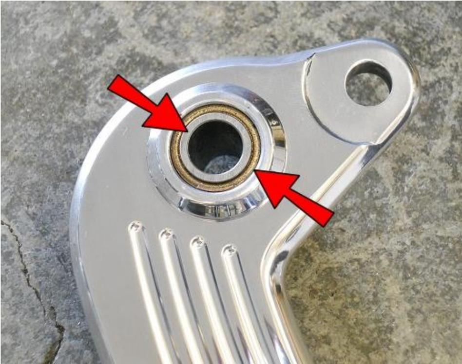
Apply some axle grease or similar, to the SLV1 and 5/8x1/2 Bronze Sleeve and insert them into the Brake Pedal, one inside the other.
