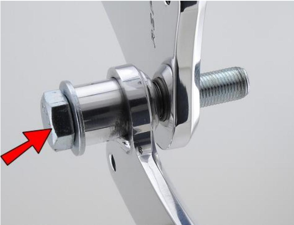
Place the 1/2-20x2.25 Bolt into the back of the Shifter Pedal and install in the 1/2" hole in the FC1-L.
