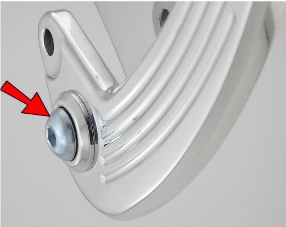
Place the 3/8-16x2 Button Head Bolt into the Brake Pedal.
