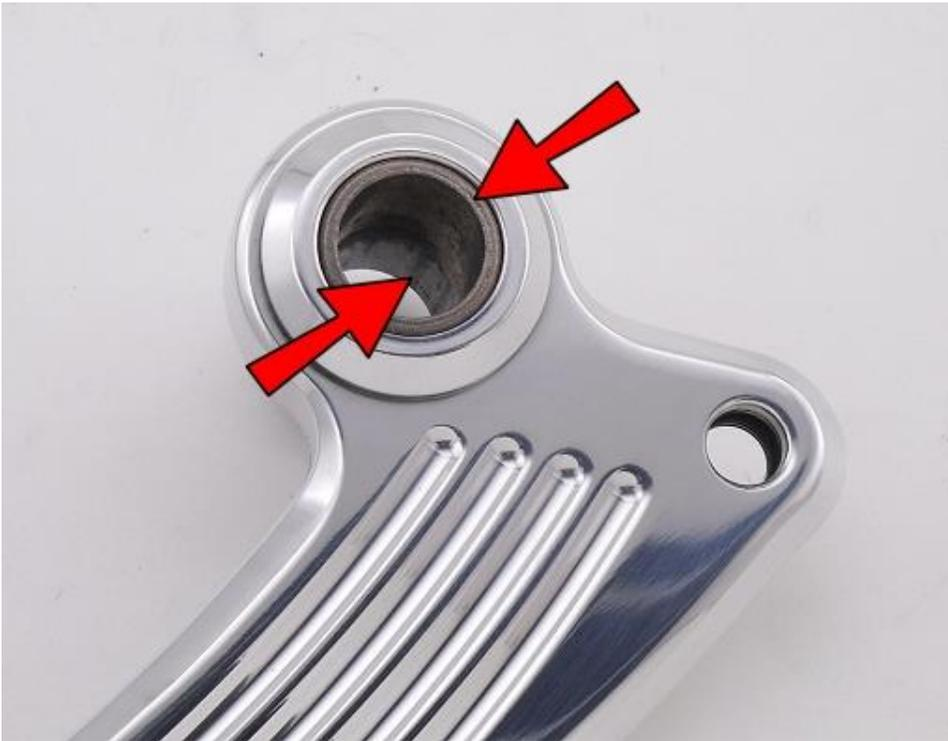
Apply some axle grease or similar, to the SPC050-2 and SPC070, then insert them into the new Shifter Pedal, one beside the other.
