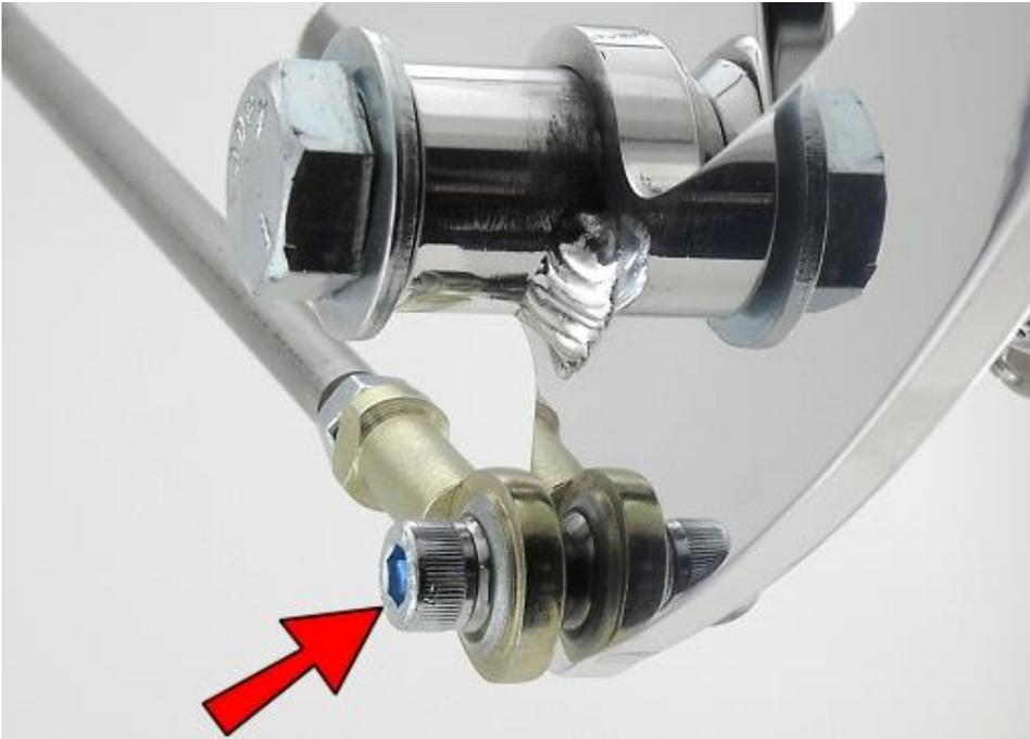
Connect the Rod End to the back side of the Shifter Pedal with an M6-1.0x25 Bolt.
