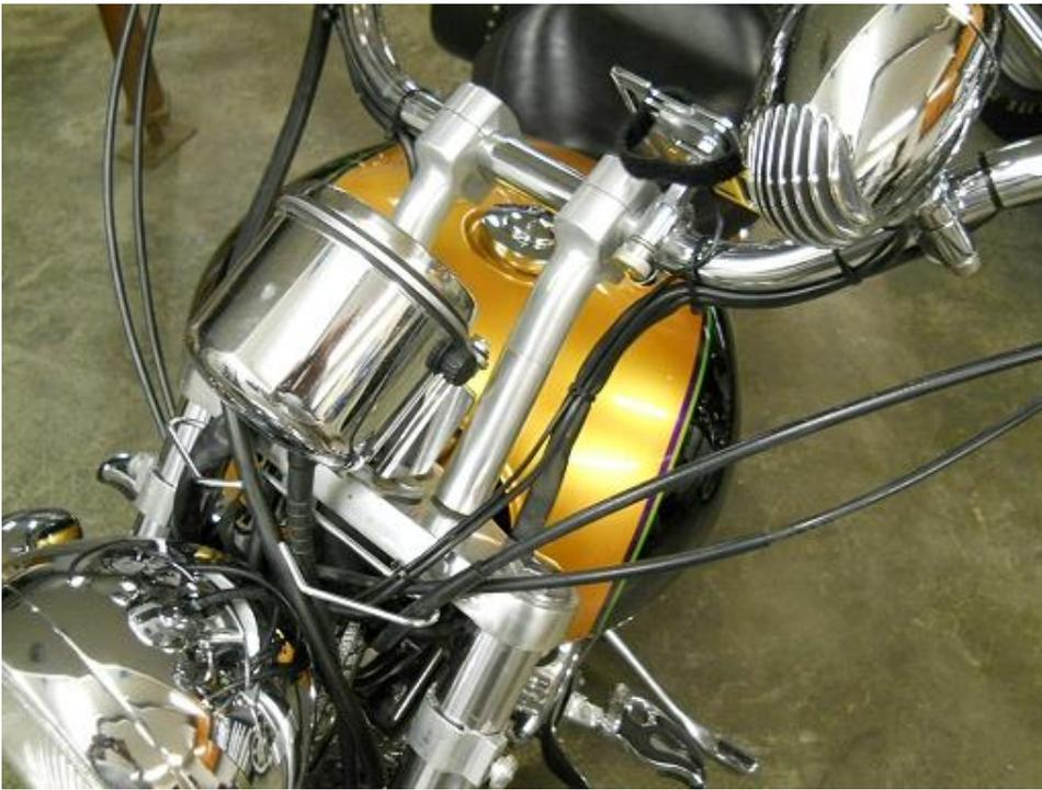
Bring the bars up into place and assure you have plenty of slack in the cables, hoses and wires.
