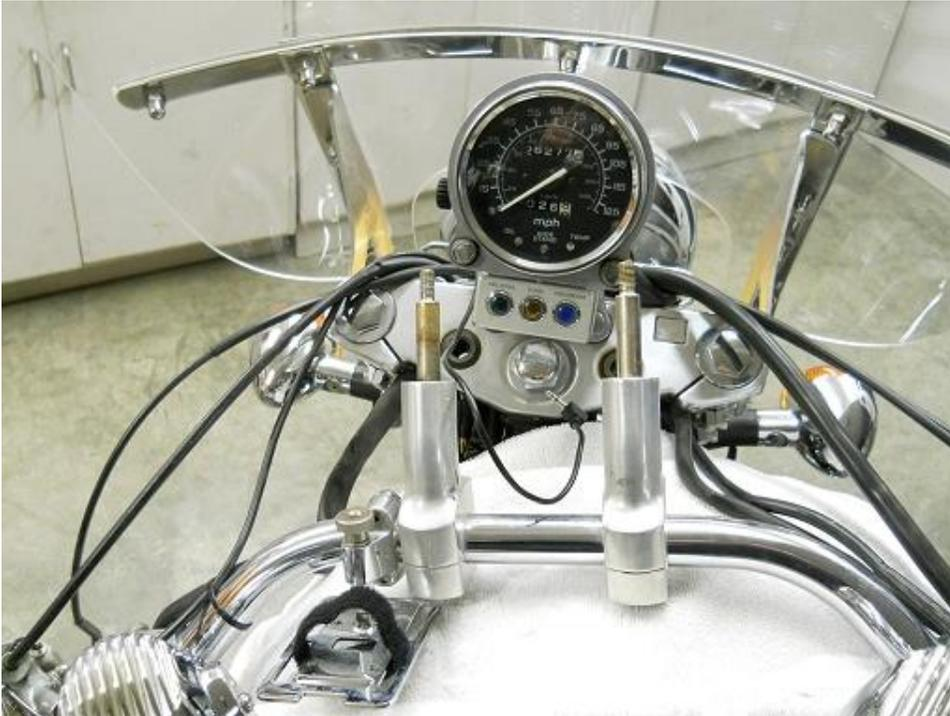
Lay a towel over your tank to protect it. Disconnect the risers from the triple tree, leaving the bars attached and lay them on the towel.
