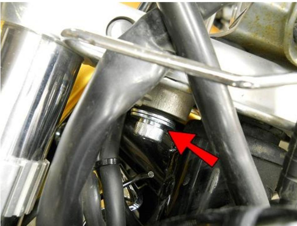
Connect the HR4's to the triple tree with the M10-1.25x70 Bolt and TWO washers (per side) provided and tighten.
