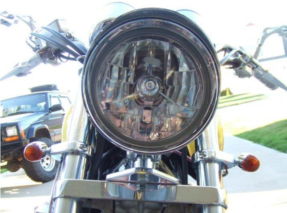
After all exposed wires are safely covered and all plugs/connectors have been reconnected, reconnect the battery. Turn ignition on and make sure the headlight works trying Hi and Low beam
