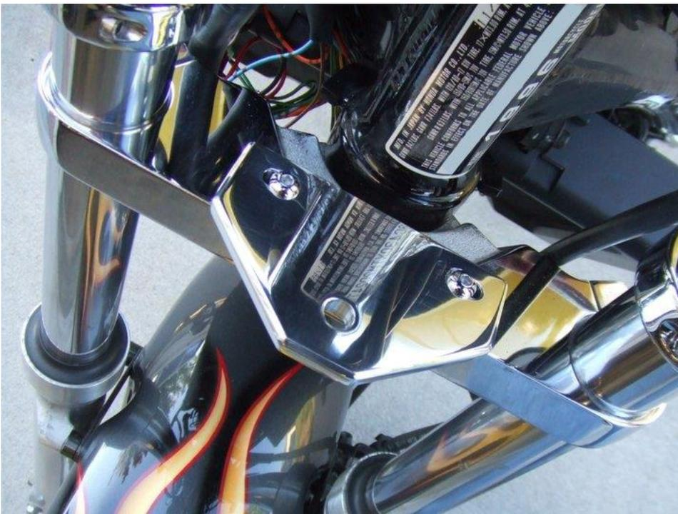
Remove the front bezel and bulb from the replacement headlight. Run the headlight wires into the small hole in the replacement headlight shell and then install onto the HM1 leaving bolt hand tight for now.
